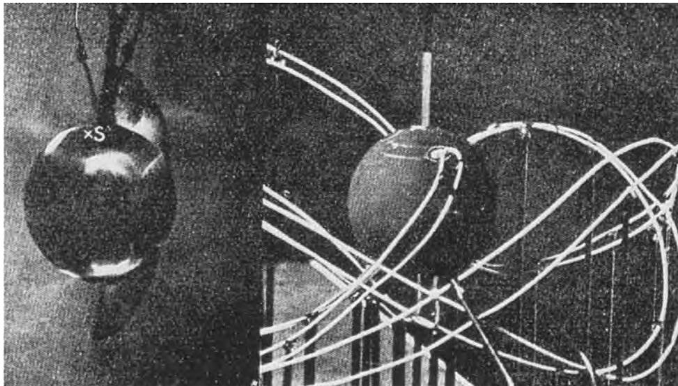
Figure 9: Birkeland's terrella with auroral zones (left) and trajectories Størmer calculated for charged particles in a dipole magnetic field (right). Agreement between the experiments and calculations is excellent. Figure is from a 1907 paper describing experiments in a cylindrical 12 litre chamber (NAPE, p. 159).
