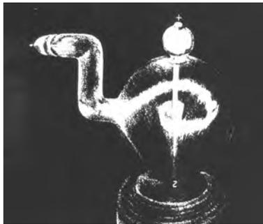
Figure 1: Photograph of Birkeland’s most successful artificial aurora produced with cathode rays inside a device that he called an auroral jar (Birkeland, 1896). The tube was placed in a large magnet. The cathode was located in a twice-bent glass tube that merged into the container. The anode was mounted in a small sphere connected by a narrow tube to the large sphere.
